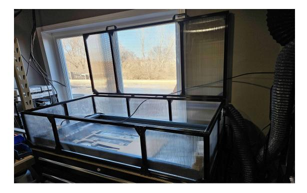
Completed Smoke Enclosure for the Laser. Quick note, if you clean off all the oil on the bottom sheet of steel used as a laser shield, you get A LOT less smoke created!!!
