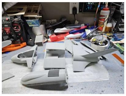
Wings and all! About 20 hours to print all the parts. Thankfully, no need to babysit. Just press go and come back a few hours later. This is a model of a DH-108 Swallow. The ruler is 15" long for a reference. It is basically a flying wing, there is no horizontal stabilizer or elevator. All control is via the wing "elevons".
