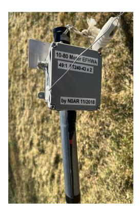
Left: This is the home-brew end fed transformer mounted on the top of the pipe.
