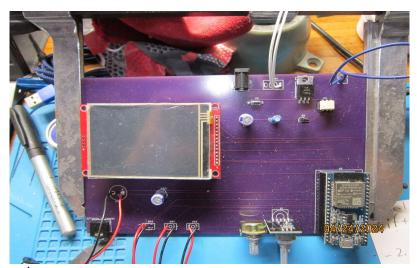
This is the QMX I built. I still need to load in the program. It should put out about 5 watts from 80m to 20m. Soldering is a little tight in places but not that bad. Notice the microphone? The designer is planning on adding SSB Phone in the future! Wow!
